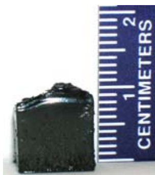
Figure 4.2. A thick 1wt% carbon black polymer created by shadow cure.
